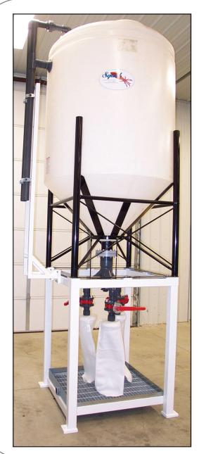
The Squid by AQUAPro Systems is a uniquely designed modular dehydration and settling system for the efficient collection of slurry. The Squid consists of a cone bottom tank of specific volume and a dehydrator manifold with valves and a series of bags collecting the concentrated slurry. The bags are easily removed for replacement and disposal.
